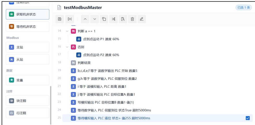
Figure 9.4.3.2-21 Wait until the AI Input Register exceeds the workflow limit.
